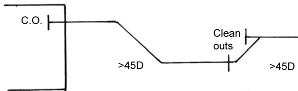
ii) Location of cleanouts for change of direction
