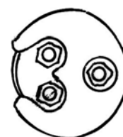
View showing the 'horse shoe' mounting plate
